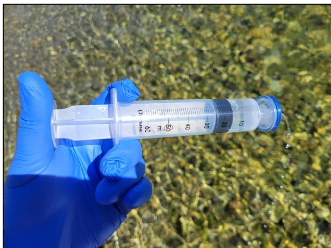
Figure 1: Syringe and filter used to collect eDNA sample.
