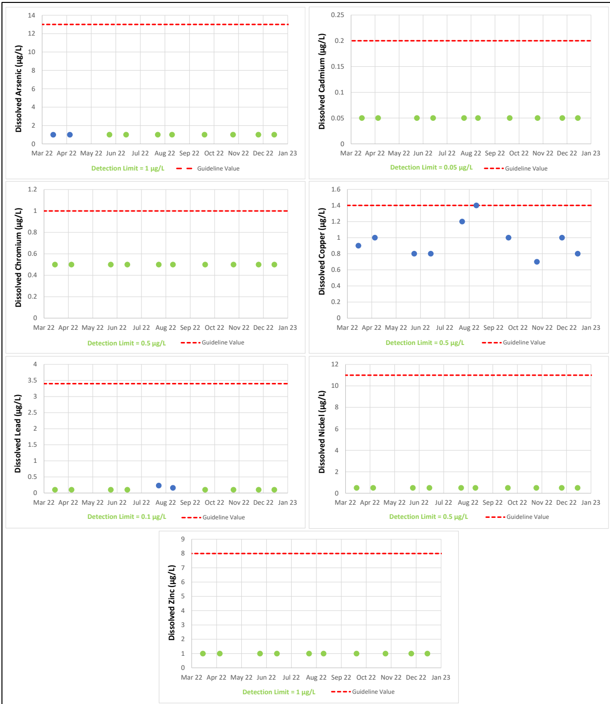
Figure 7: Dissolved metal results for arsenic, cadmium, chromium, copper, lead, nickel and zinc for the Opuha River below the Downstream Weir and comparison to guideline value (-----). Green dots (■) indicate values less than the detection limit and blue dots (■) indicate values above the detection limit.
